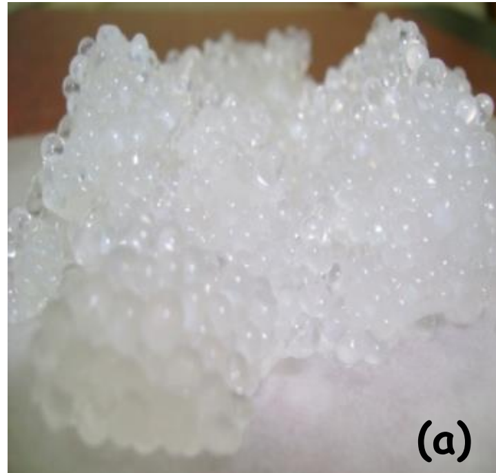
Biopolymer Q/X, 50/50 and 5% crosslinker (a) hydrogel and (b) xerogel
